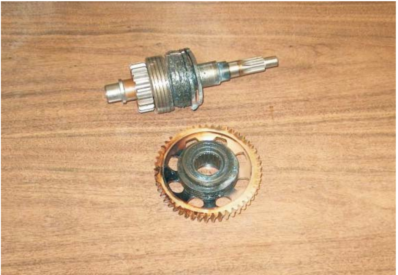
STARTER NOT OVERHAULED / CLUTCH SPRING FAILED TO RELEASE
