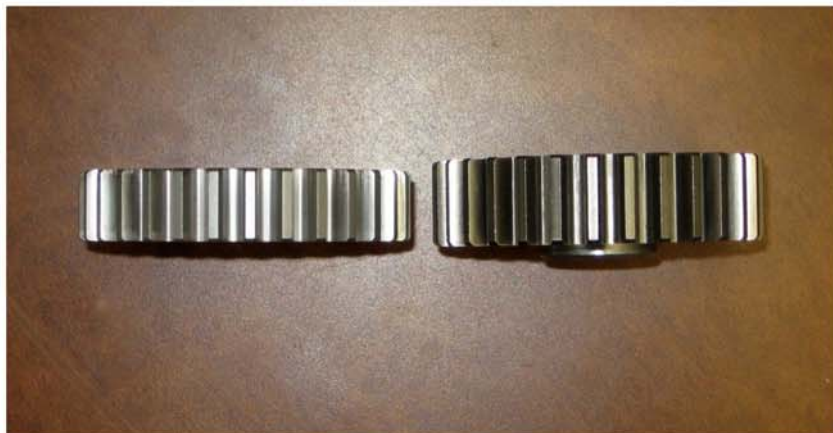
The gear on the left is the old style while the gear on the right is the 657175 part number configuration. The increased height in the new gear is very obvious. The gear bolts hitting the Classic starter adapter is very possible and clearance must be checked.
