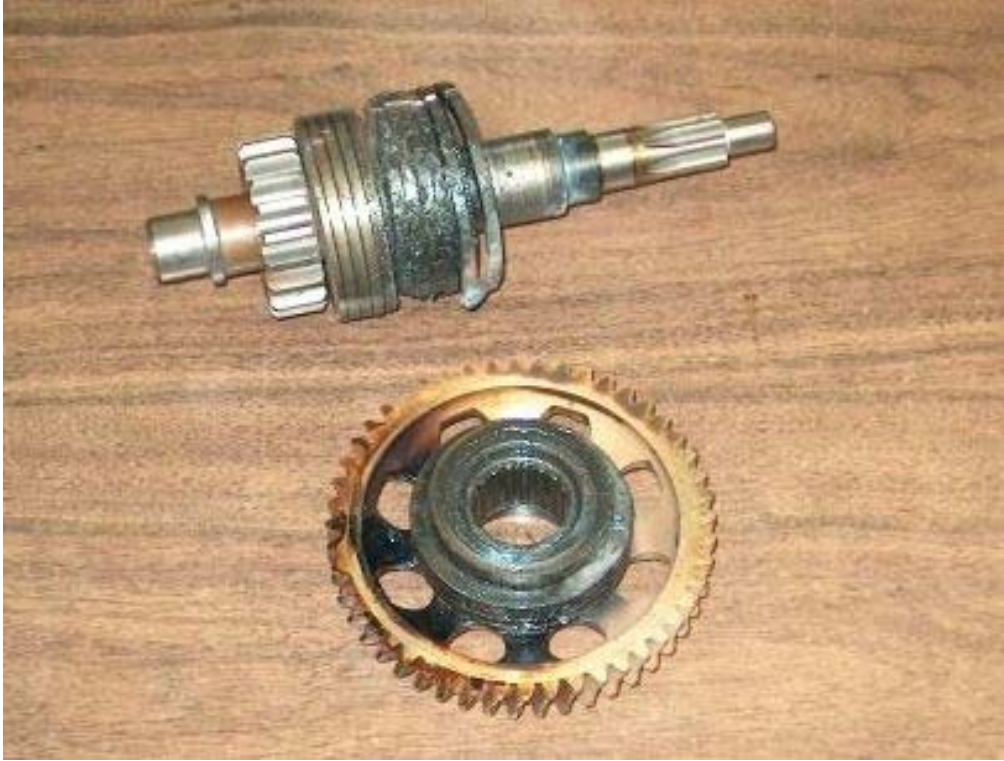
STARTER NOT OVERHAULED / CLUTCH SPRING FAILED TO RELEASE
